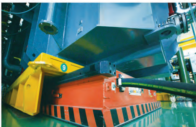
480t air cushion crane
