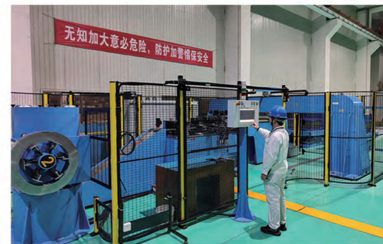
Automatic core stacking machine
