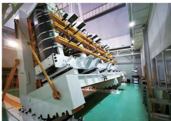
300t core stacking & overturning platform
